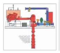
NFPA #20 requires the use of a vertical turbine on systems operating under a static suction lift condition requirement. A-C Fire Pump Systems offers the complete pre-packaged system, pump, driver, controller, flow measuring device, control valves, check valves, sensing lines and power distribution panel. This system requires one electrical connection and a water supply. It's ready to provide immediate, reliable fire protection.
